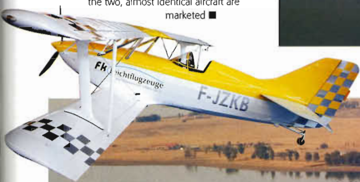
The Fk12 Comet ultralight biplane: 'demonstrated ultimate load' +9/-3.5g..
