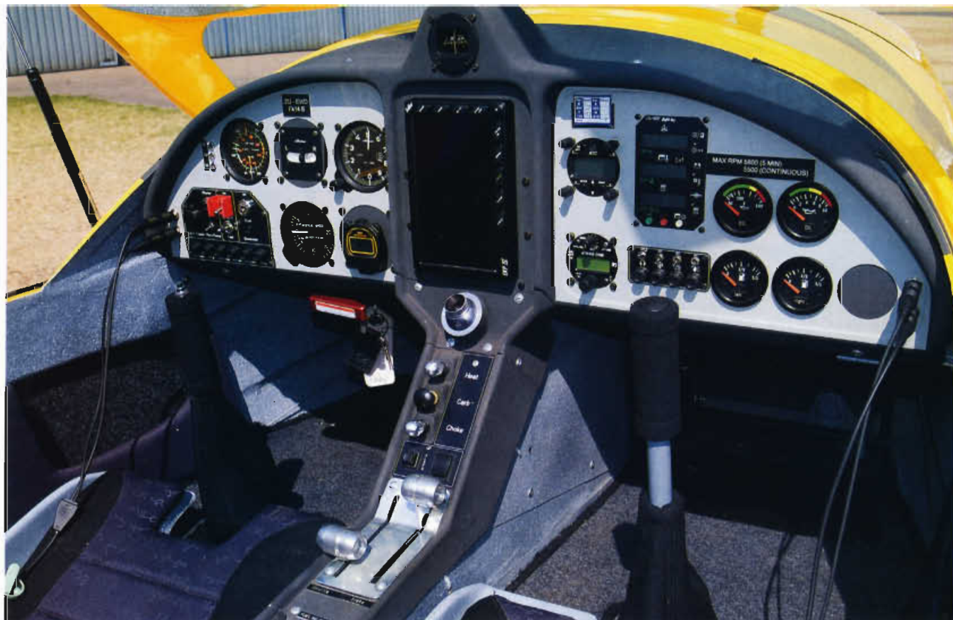
Nicely kitted out in the round-instrument tradition, the Fk14 nevertheless features an AvMap EXP-IV navigation unit (centre panel) and a UL MK engine management system (right-hand sub panel). From bottom, centre console mounts paired throttle and brake levers, electric flap switch, choke, carb & cabin heat
