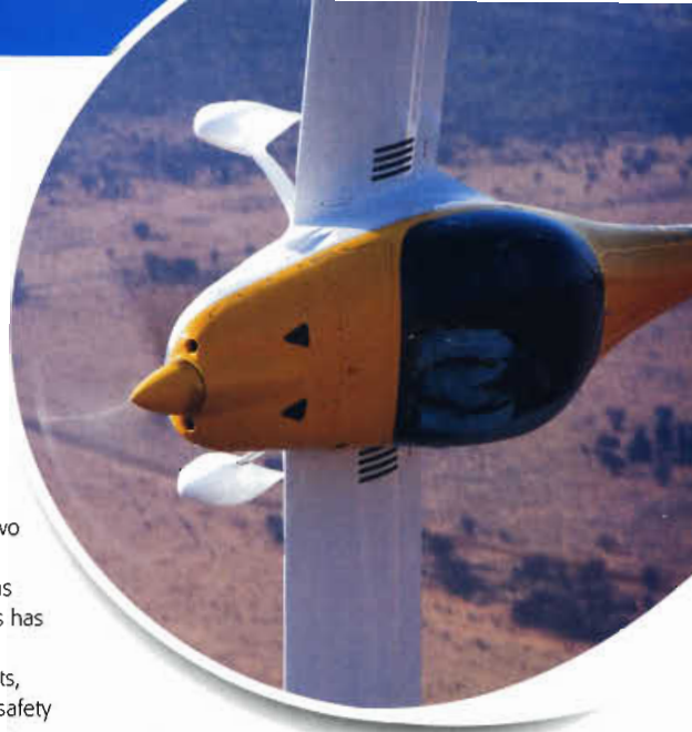
The slippery lines of the Polaris run from the spinner back, the liquid-cooled Rotax 912 being tightly cowled, with minimally-sized intakes
