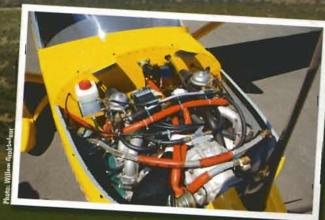
Right: Rotax power (what else) for the FK 9. The cowls are easily removed to reveal a smart and clean engine bay.
